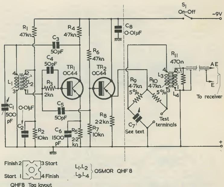
Fig. 1. The circuit of the capacitance measuring instrument. The bridge circuit proper (R<sub>9</sub>, R<sub>10</sub>, C<sub>7</sub> and the "test terminals") is that initially employed in the prototype
