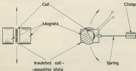
Fig. 2. The basic method of operation of the vibration transducer. The coil swings between the two magnets
