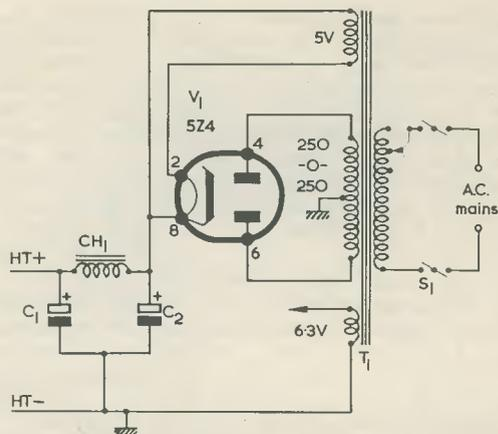
Fig. 2. A suitable power supply for the receiver
