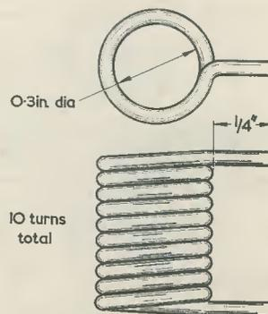
Fig. 5. Construction of the heater chokes L<sub>8</sub> and L<sub>9</sub>
