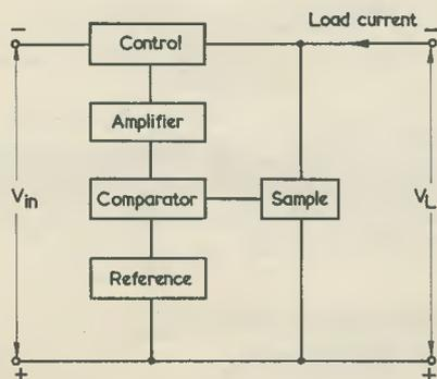
Fig. 1. Block diagram of a regulated power supply
