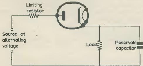
Fig. 258. Inserting a limiting resistor to prevent excessive peak currents in the rectifier
