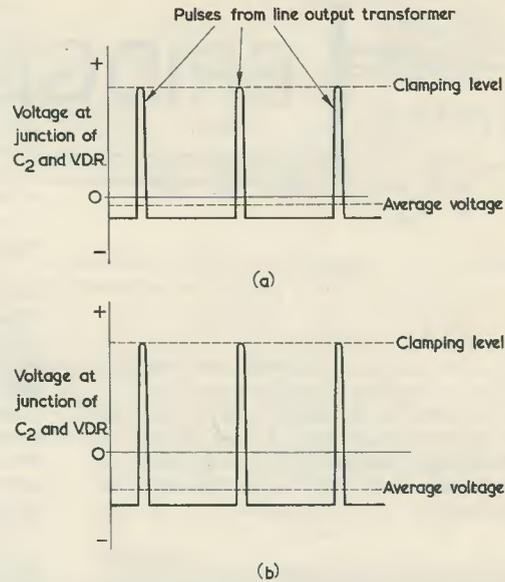
Fig. 12 (a). The v.d.r. of Fig. 11 holds the positive tips of the flyback pulses at clamping level. The average voltage of the waveform, at the junction of  $C_2$  and the v.d.r., is then negative of chassis
