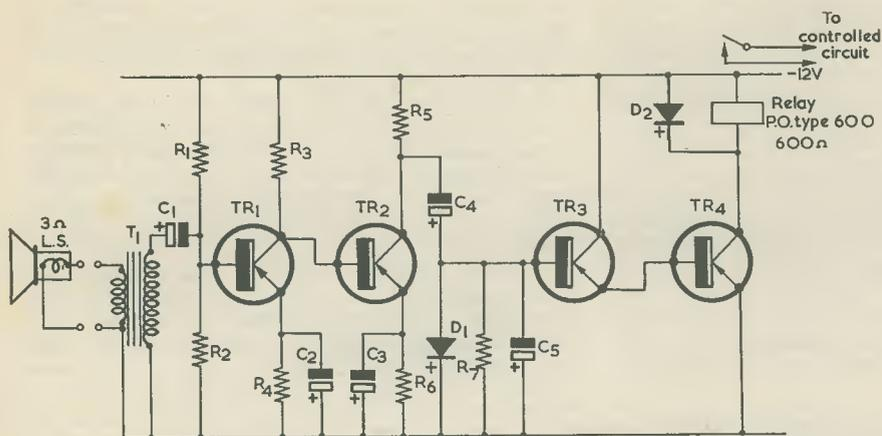
Fig. 1. The circuit of the sound-operated switch. The loudspeaker is employed as a pick-up microphone
