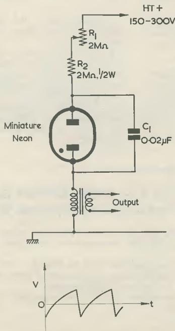
Fig. 9. A simple neon oscillator. The output transformer may have a ratio between 1:4 and 1:5
