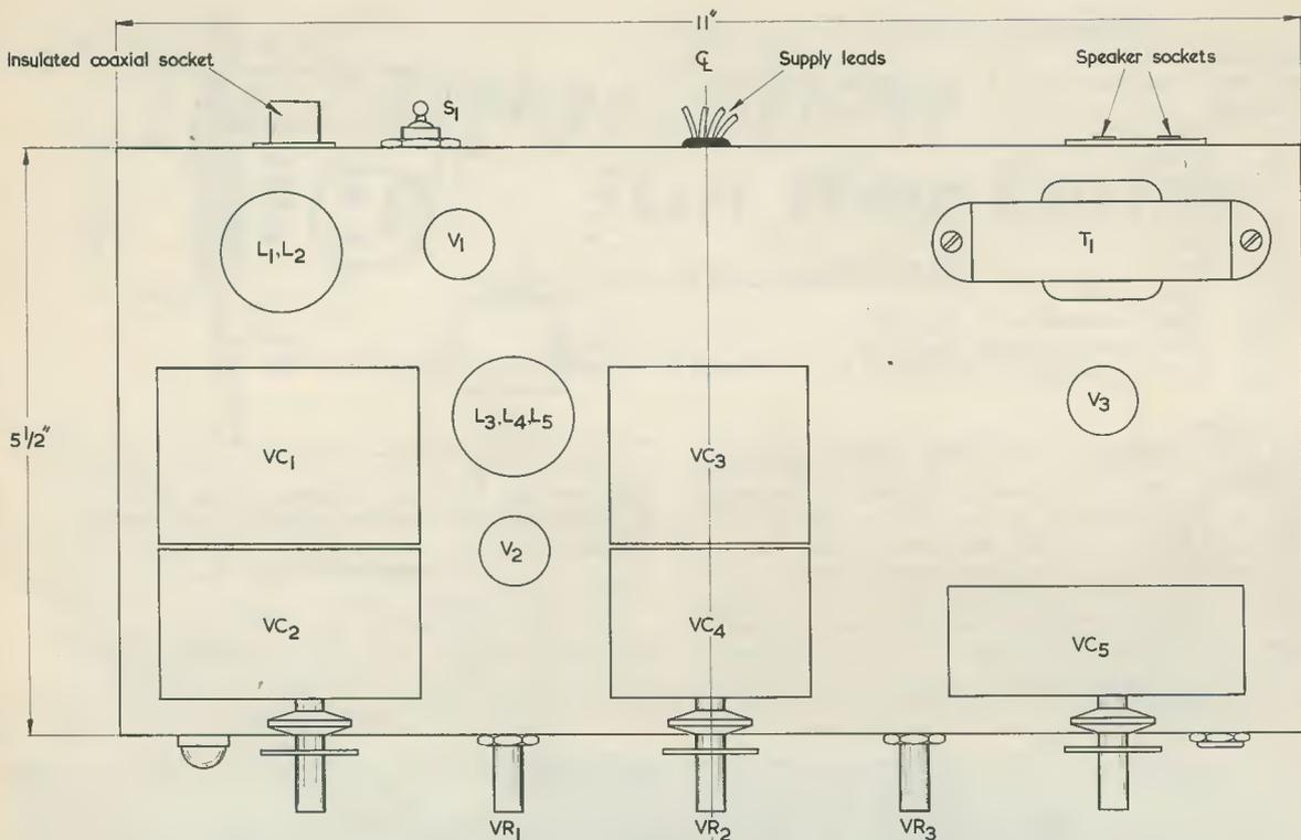
Fig. 3. Outside dimensions and above-chassis layout. The depth of the chassis is  $2\frac{1}{2}$  in. The aerial and r.f. coils appear, in their screening cans, above the chassis
