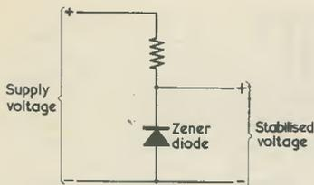
Fig. 1. Employing a zener diode to obtain a stabilised voltage. The voltage across the zener diode remains very nearly constant despite changes in supply voltage
