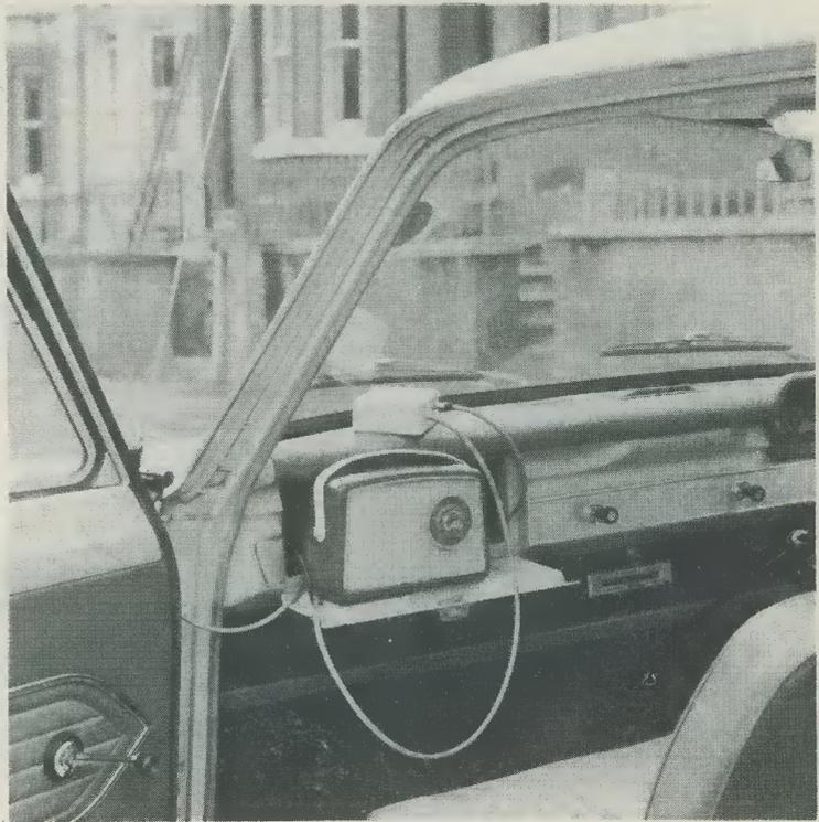
The “King Karad” booster in use with a car aerial and transistor radio. This little device, which is shown here above the radio, offers a minimum of 20dB amplification without tuning over the entire medium and long wave bands, together with correctly designed matching to both the aerial and the receiver
