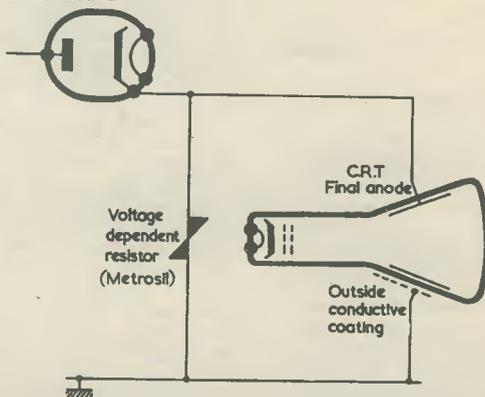
Fig. 5. Employing a Metrosil to improve the regulation of the e.h.t. voltage applied to the final anode of a c.r.t. (Metrosils are manufactured by Associated Electrical Industries Ltd.)
