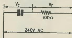
Fig. 2. Measuring capacitance by the voltmeter method
