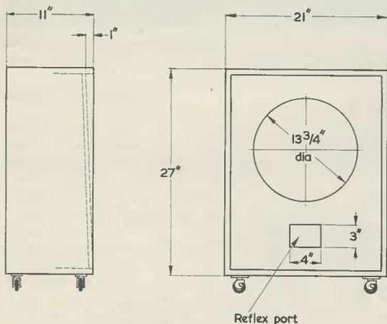
Fig. 1. A suitable reflex enclosure which may be home-constructed
