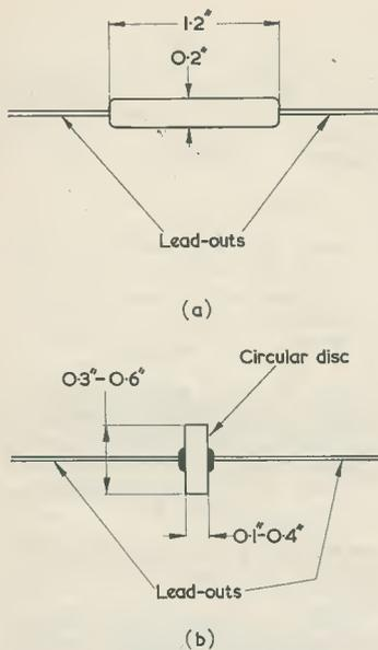
Fig. 6. Small voltage dependent resistors may appear in a similar form to normal resistors (a), or to disc ceramic capacitors with the leads protruding from the centre of the surfaces (b). The dimensions given here are representative and are only intended to give a general idea of size
