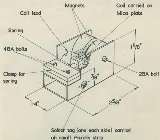
Fig. 3. The dimensions of the vibration transducer constructed by the writer
