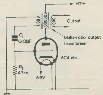
Fig. 10. A blocking oscillator. The manner in which a suitable transformer may be obtained is discussed in the text
