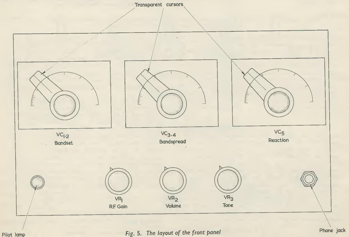
Fig. 5. The layout of the front panel
