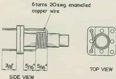
Fig. 3. The construction of  $L_2$
