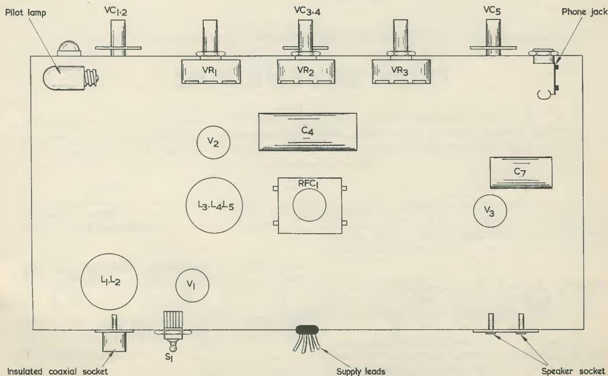
Fig. 4. The positions taken up by the principal components below the chassis
