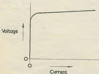
Fig. 2. The voltage-current characteristic of a typical zener diode
