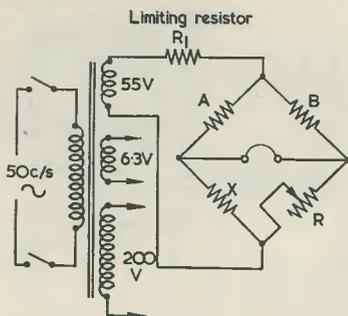
Fig. 13. Inserting a limiting resistor between the a.c. source and the bridge
