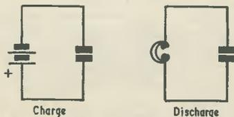
Fig. 1. A simple charge and discharge test
