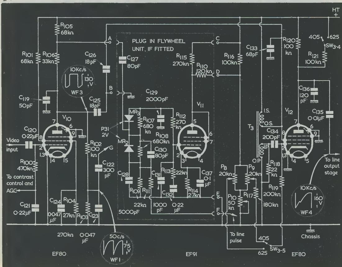
Fig. 30. This circuit section from a dual-standard set shows the sync separator, the flywheel controlled line sync and the line oscillator at valves V<sub>10</sub>, V<sub>11</sub> and V<sub>12</sub> respectively
