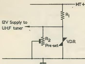
Fig. 10. Obtaining a stabilised 12 volt supply from the h.t. line of a television receiver for a transistorised u.h.f. tuner. Representative component values are  $R_1$  10k $\Omega$ , and  $R_2$  15k $\Omega$
