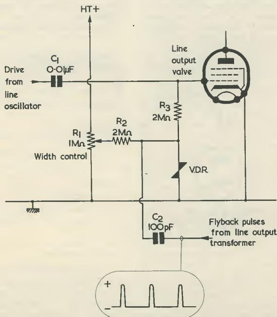
Fig. 11. A basic circuit, with representative component values, illustrating the use of a v.d.r. for picture width stabilisation
