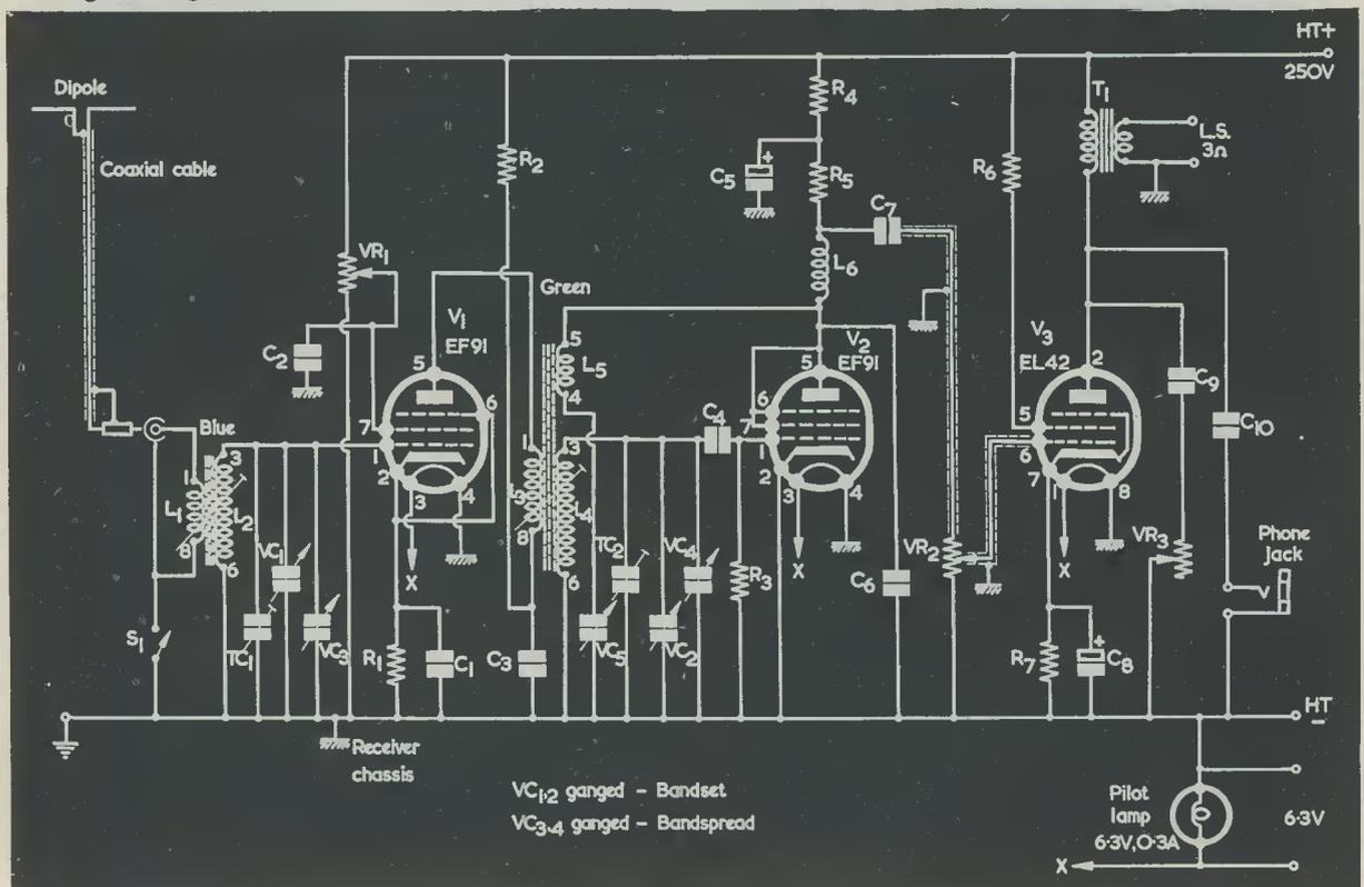
Fig. 1. The circuit of the "Zephyr". If a normal aerial is employed, this is connected to the centre contact of the coaxial socket and  $S_1$  is closed
