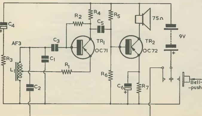
Fig. 1. The circuit of the single-ended unit
