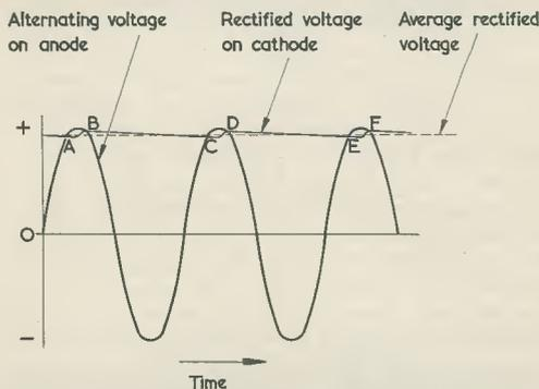
Fig. 259. If the load resistance is made very high, the reduced load current causes the average rectified voltage to closely approach the peak value of the applied alternating voltage
