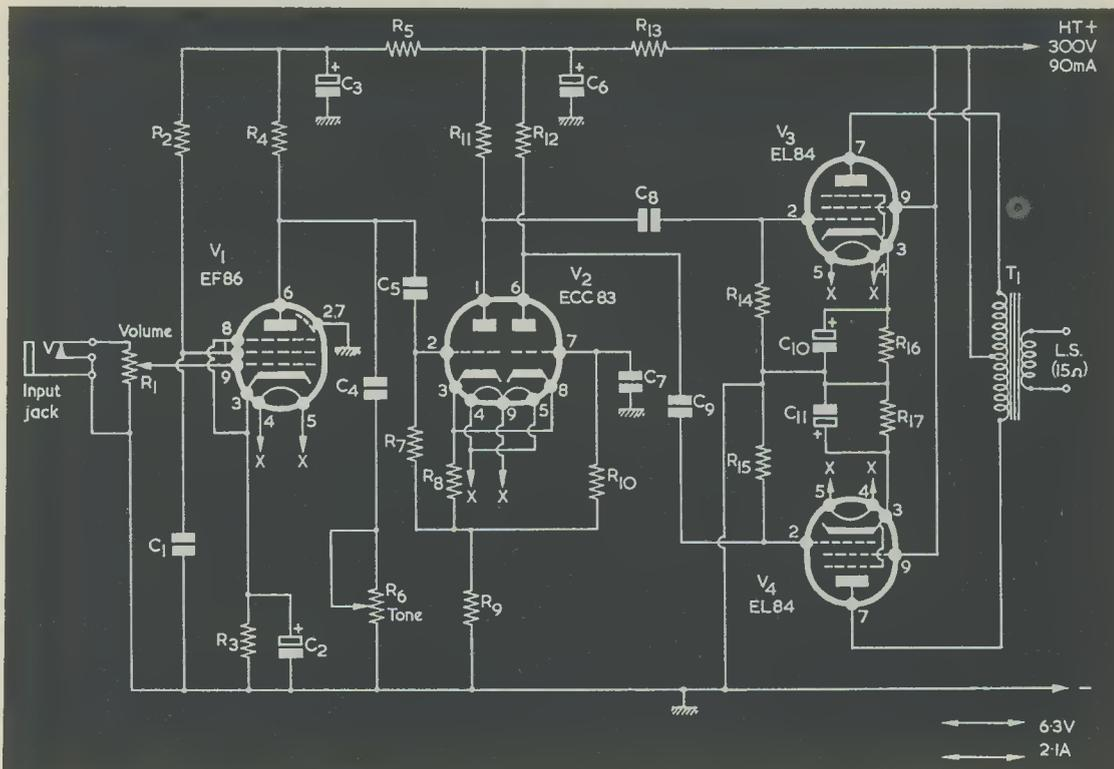
Fig. 2. Circuit for a 17 watt amplifier for use with the bass guitar. In the event of instability, 1k $\Omega$  series grid stoppers may be inserted close to the grids of V<sub>3</sub> and V<sub>4</sub>
