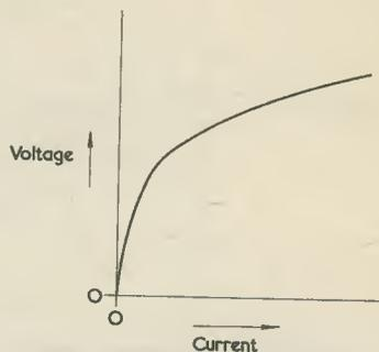
Fig. 4. The voltage-current curve of a voltage dependent resistor. The existence of a relatively flat top makes it fairly similar to the zener diode curve of Fig. 2
