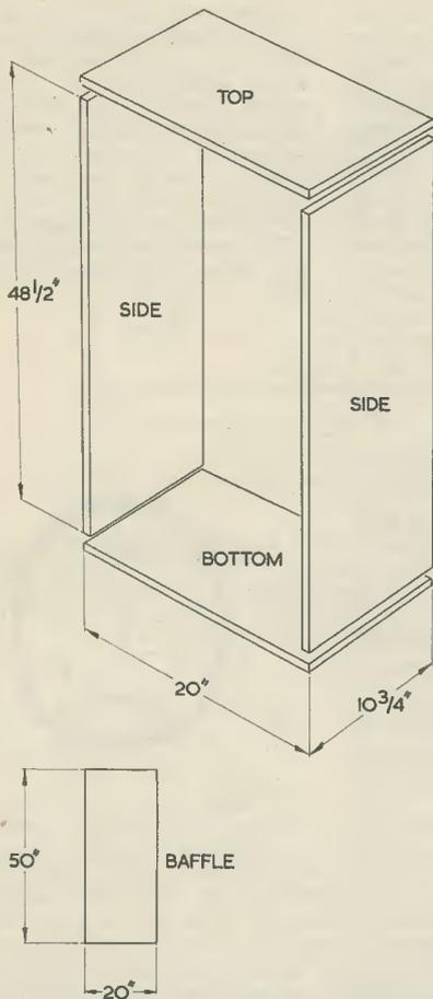
Fig. 2. Dimensions of the front, top, sides and bottom of the enclosure. The back, which is discussed in the text, has the same dimensions as the front baffle
