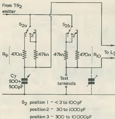
Fig. 2. A suggested bridge circuit which enables measurements to be made from less than 3pF to 10,000pF. The resistors should be 5% types or better, according to the degree of agreement required between the ranges covered by  $C_7$ . The trimmer shown in dotted line may be helpful if there is a wide unbalance in stray capacitances to chassis at the output terminals of the bridge
