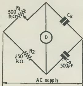
Fig. 3. The capacitance bridge
