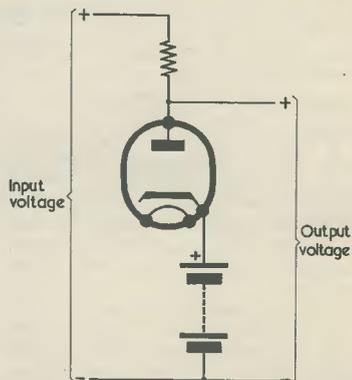
Fig. 3. Using a diode and battery as a clamping device. The output voltage remains slightly in excess of battery potential for all input voltages above that of the battery
