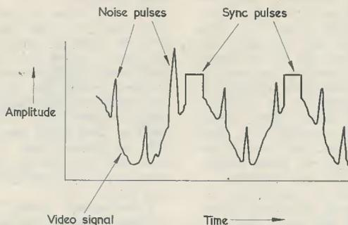
Fig. 31. As an interference pulse rises in a positive direction on the negative picture signal on the 625 line standard, the use of flywheel controlled line sync is desirable on this standard to avoid random "firing" of the line oscillator and consequent ragged vertical edges on the picture
