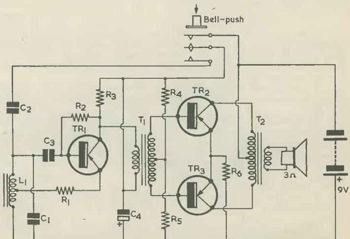
Fig. 3. The circuit of the alternative push-pull version
