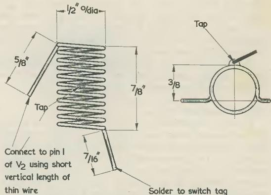
Fig. 4. The oscillator coil L<sub>3</sub>. References to V<sub>2</sub> and the switch tag are with respect to the layout diagram of Fig. 9, which will be published next month
