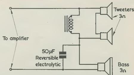
Fig. 1. The crossover network employed by the author. The inductor is the  $3\Omega$  secondary of a small output transformer, whilst the capacitor is a  $50\mu\text{F}$  reversible (i.e. non-polarised) electrolytic component
