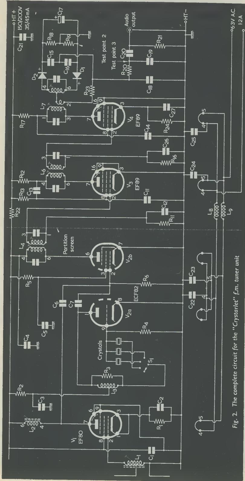
Fig. 2. The complete circuit for the "Crystarlet" f.m. tuner unit
