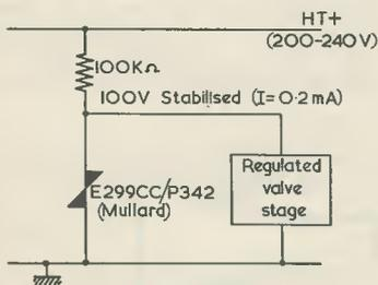
Fig. 7. An example showing the use of a v.d.r. to regulate the h.t. voltage fed to a stage in valve equipment. Despite variations in h.t. potential from 200 to 240 volts, the change in the potential applied to the valve stage is only of the order of 7 volts
